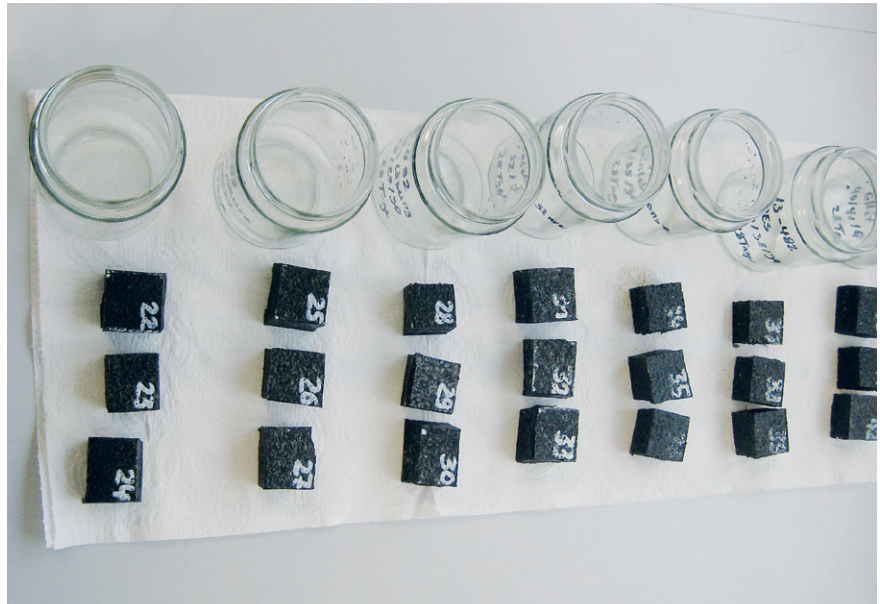
Figure 9: Test samples after the acid test
